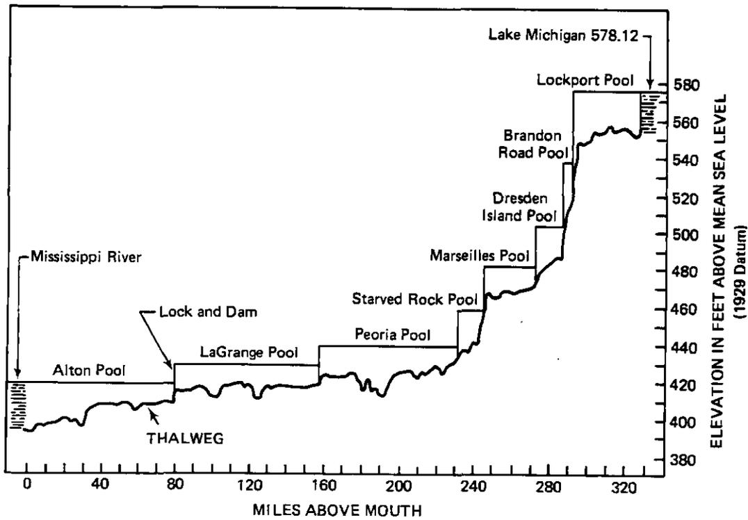
Figure 2. Profile of the Illinois Waterway.
