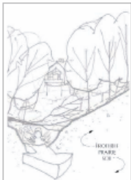
Figure 15. Image shows the collective contribution of concentrated rainwater from streets and the cutting the soft glacial soils.
