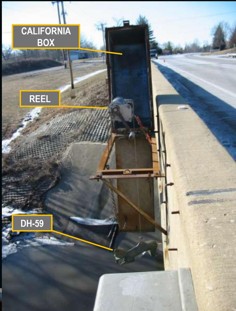
Weekly samples are taken at a fixed location over the thalweg of the main channel using a California-style sediment box that houses a cable, reel, and DH-59 depth-integrated sampler
