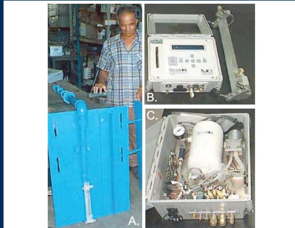
Figure 8. Double Bubbler Pressure Differential Instrument (a) in-stream components before installation, (b) controller and orifice bar, and (c) air compressor and tank assembly. Figures 8b and 8c courtesy of Design Analysis Associates, Inc.
